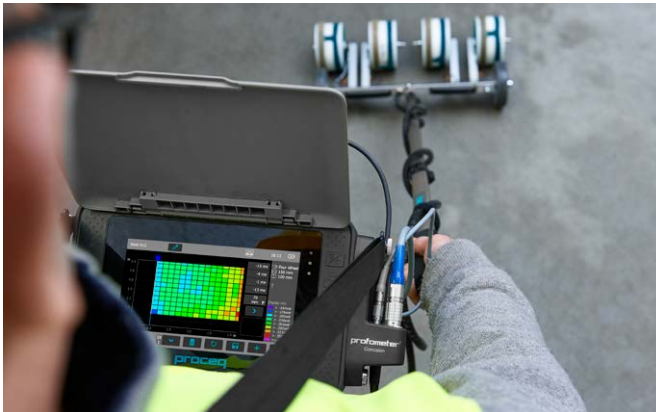
Profometer Corrosion with a 4 wheel electrode
