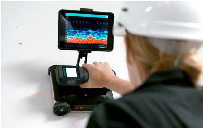
Proceq GPR Live probe combined with the device tablet holder
